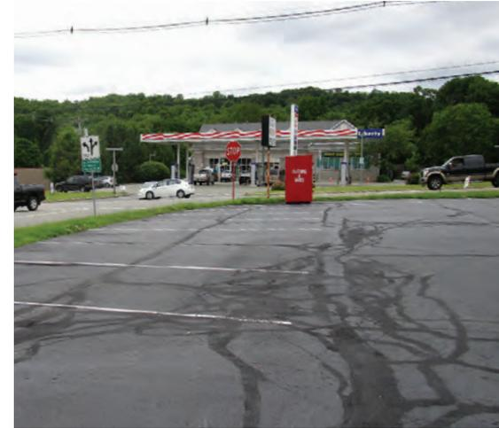
Areas of the parking lot can be retrofitted with porous pavement to capture stormwater runoff from the parking lot. A preliminary soil assessment suggests that the soils have suitable drainage characteristics for green infrastructure.
